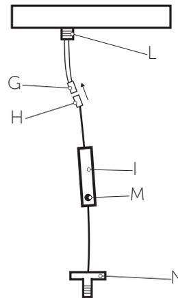
Screw the tube I to the threaded rod L. Finally tighten the Allen screw M in the tube I in order to lock the electric cable.
